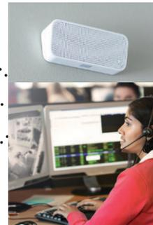
When the alarm centre receives an alarm, the operator opens an audio connection. You can cancel the alarm by giving your cancellation code. If the alarm centre operator confirms that the alarm was caused by a break-in or a fire, this information is relayed immediately to the police or rescue services.
